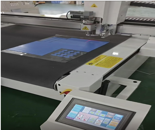
CNC proofing machine, no need to make molds, saving mold costs for customers
